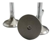
Inconel (in·kuh·nel) valves are made of a nickel-based super alloy with high corrosion and oxidation resistance. These valves are very robust in high temperature environments and help provide creep resistance.
